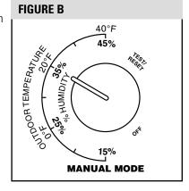
hear the solenoid valve "click on." Next, slowly turn the dial counter clockwise until you hear the solenoid valve "click off." At this point, read the RH on the dial. This will be very close to the actual RH in your home. (See Figure B)
