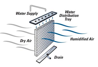
The humidifying principle of all Aprilaire Humidifiers uses the introduction of humidity in the form of water vapor to prevent minerals from entering the air stream in the home. Water is supplied to the distribution tray, allowing it to flow evenly across the water panel. The resulting humidified air is distributed throughout the entire home.
